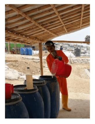
The faecal sludge treatment site is designed with the primary objective of pathogen elimination. It consists of lime stabilisation for pathogen elimfination, unplanted drying beds for solid liquid separation and dewatering and a sludge drying area.
